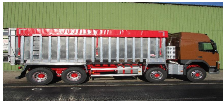
High sided Garstang type bulker body
