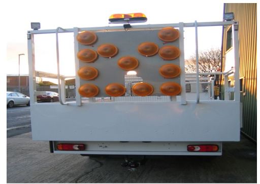
Aluminium planked tail door with traffic management light arrow board
