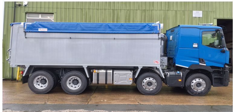
High sided aluminium planked tipping body with Dawbarn sheeting system
