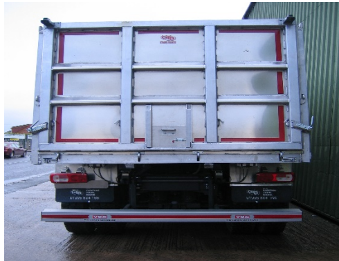
Air lock / unlock one-piece tail door with manual opening hatch at floor level
