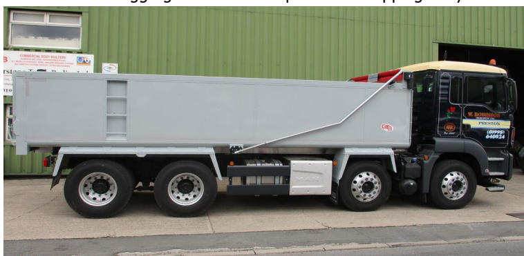
8-wheeler insulated tipping body with Transcover side arm sheeting system
