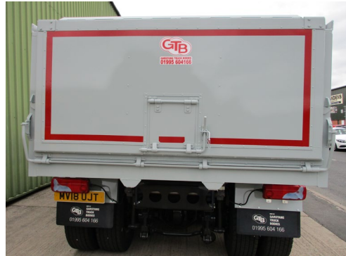
One-piece manual opening tail door with one manual opening hatch at floor level
