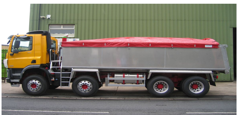
8-wheeler insulated tipping body with Harsh electric sheeting system
