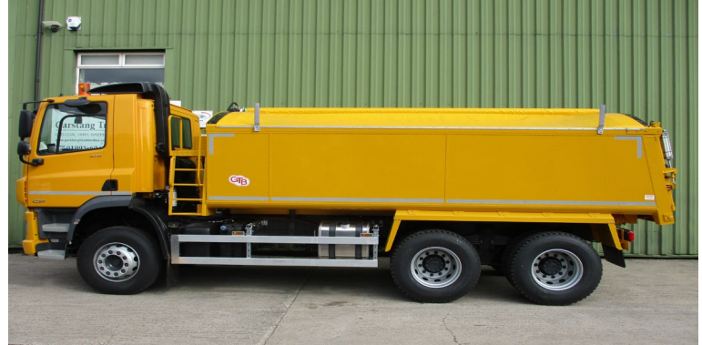
6-wheeler insulated tipping body with Dawbarn electric sheeting system
