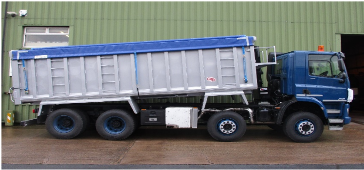
Bulker body with manual opening sheeting system
