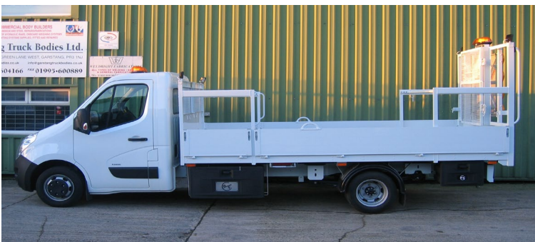
Non-tipping traffic management type drop sider body
