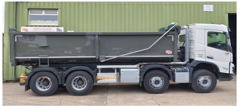
Hardox type tipping body with Transcover side arm sheeting system
