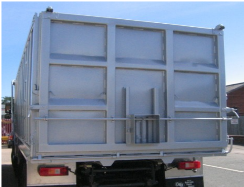
One-piece tail door with rack and pinion hatch
