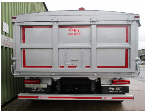
One-piece tail door hung from header beam with manual opening hatch
