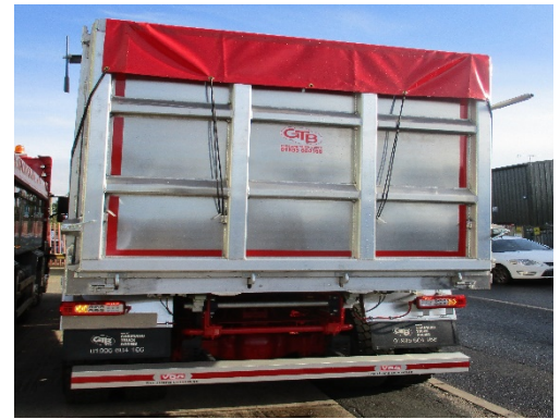
Air lock / unlock one-piece tail door
