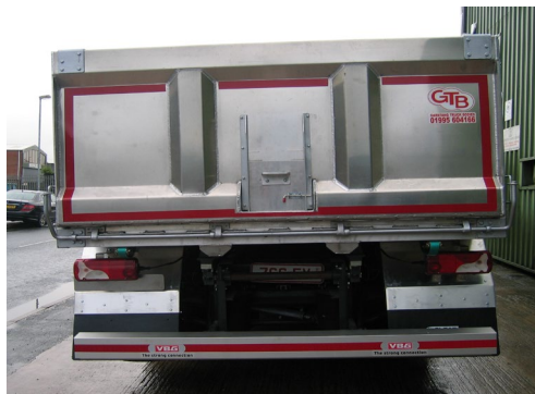
One-piece manual opening tail door with manual opening hatch
