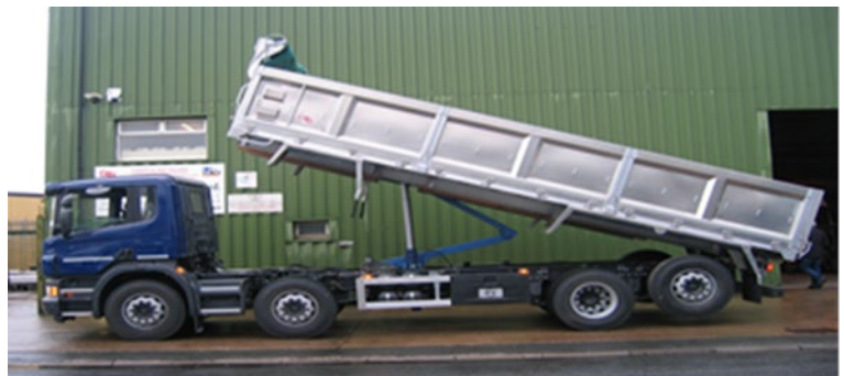
Triple drop sided body with underfloor tipping ram
