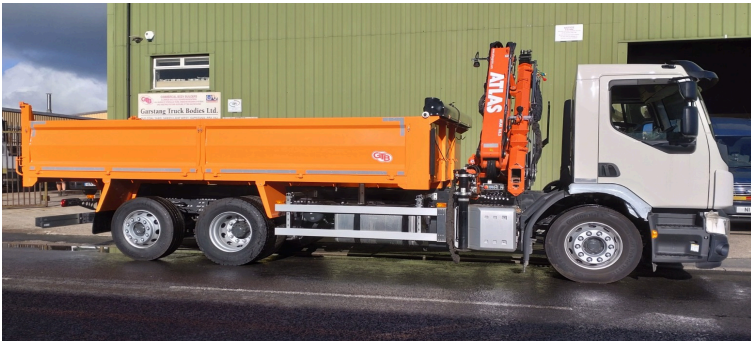
Aluminium double drop sided body with Hardox floor
