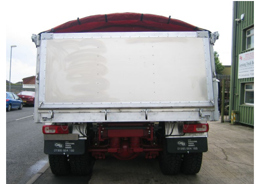
One-piece air lock / unlock tail door
