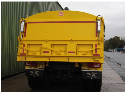
Air opening split tail door with 3 manual opening hatches at floor level
