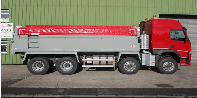
8-wheeler insulated tipping body with Dawbarn electric sheeting system
