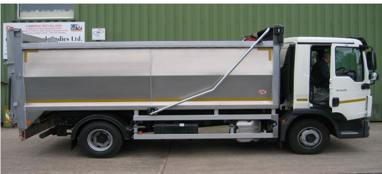
Animal waste type body with Transcover side arm sheeting system
