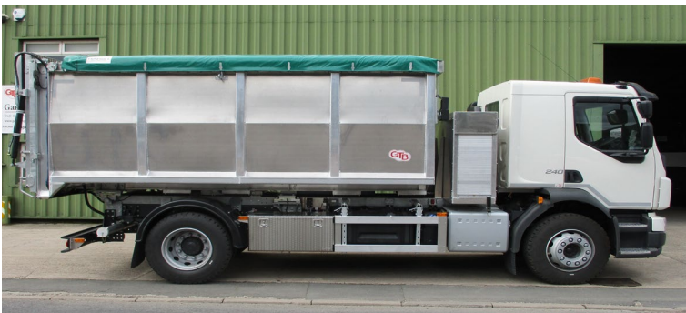
Animal waste type tipping body with Harsh sheeting system
