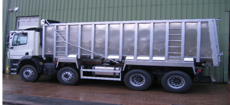
Bulker body with Transcover side arm sheeting system
