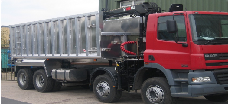
Bulker body with HIAB crane
