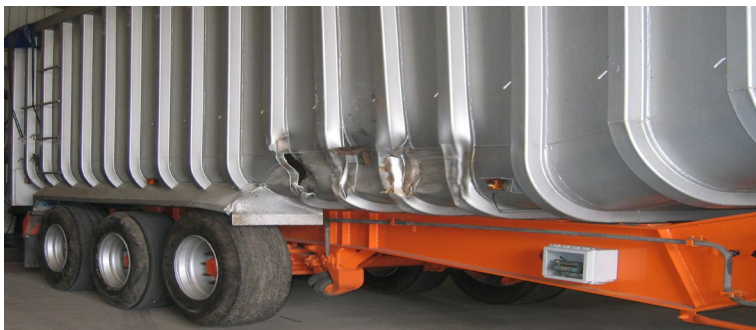
Trailer brought in with damaged side
