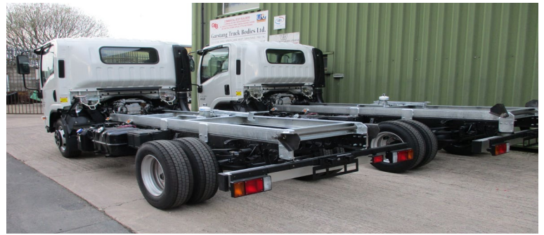
Subframes manufactured and fitted
