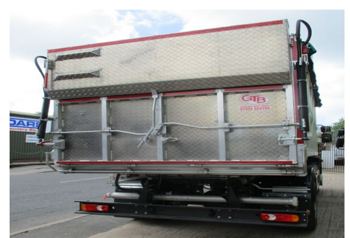
Top hung tail door with ability to open as ramp with hydraulic rams operated by wander lead
